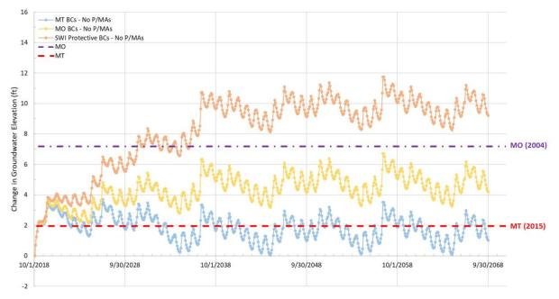
Figure ES-3. Comparison of Groundwater Elevation Changes Under "No Project" Scenario with Various Boundary Conditions and 2030 Climate Condition, Marina-Ord Area WBZ
